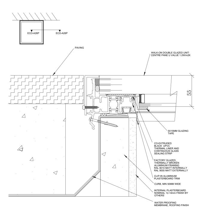
CONCENTRATED LOAD MUST NOT EXCEED 3600 N AND UNIFORM DISTRIBUTED LOAD MUST NOT EXCEED 5000 N/m<sup>2</sup>
