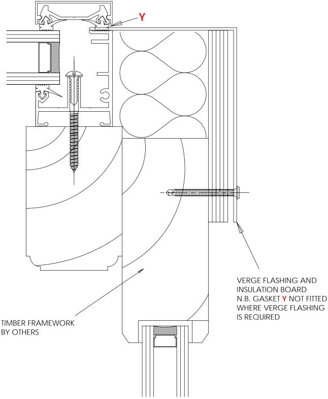
Eaves perimeter detail Cad Code WF05
