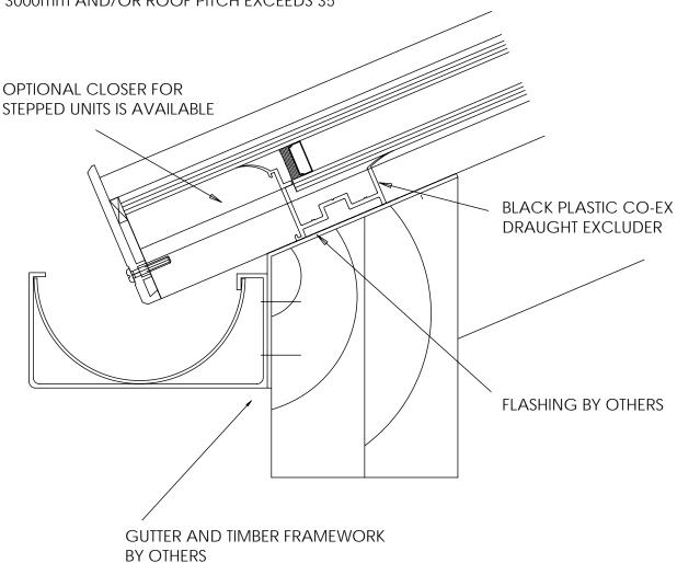
Top mono-pitch detail Cad Code WF06
